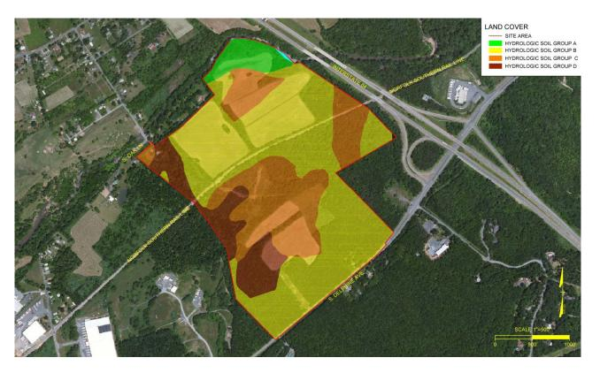
Figure 16: Map of Soil Survey Data by Hydrologic Soil Group
