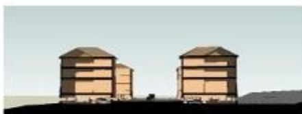
Phase 1 Construct new 3 story buildings on columns with parking below in the flood-prone area.
